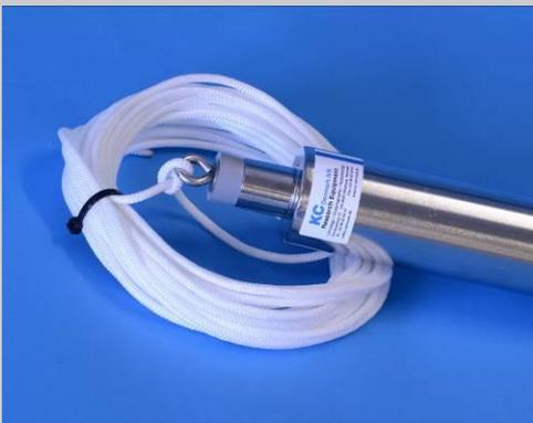
The inner of the sample tube has a stainless steel weight, 650 g for improving the deployment.
