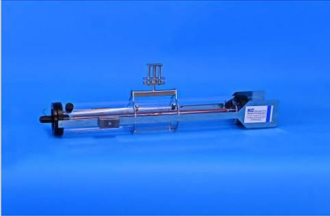
Van Dorn water sampler with integrated direction fin.
