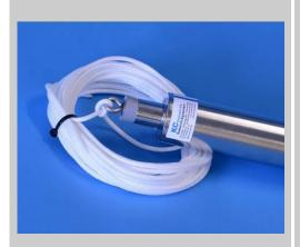
The inner of the sample tube has a stainless steel weight, 650 g for improving the deployment.
