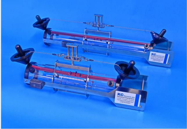
The water sampler is based on the Van Dorn design.
